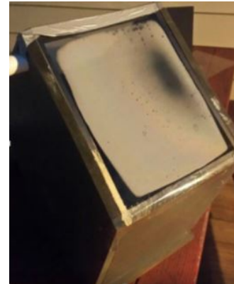
Figure 3: Shown here is condensation which has formed on the Plexiglas roof of the prototype condensate collector.
