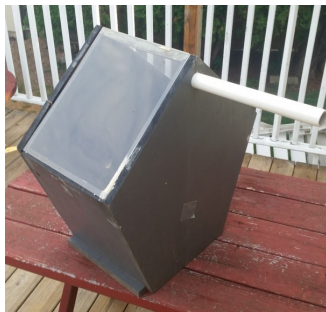
Figure 2: Picture of the completed prototype condensate collector.
