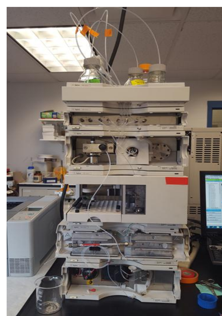
Shown above is the Agilent 1100 Series high-performance liquid chromatography instrument used for analysis
