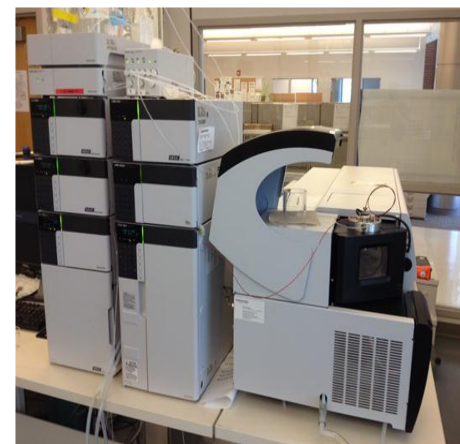
Shown above is the high performance liquid chromatography/triple quadrupole mass spectrometry instrument used at the Connecticut State Crime Lab for analysis.
