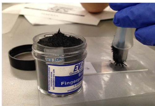
Figure 2: Gently brushing the magnetic fingerprinting over the fingerprint residue with the magnetic wand.
