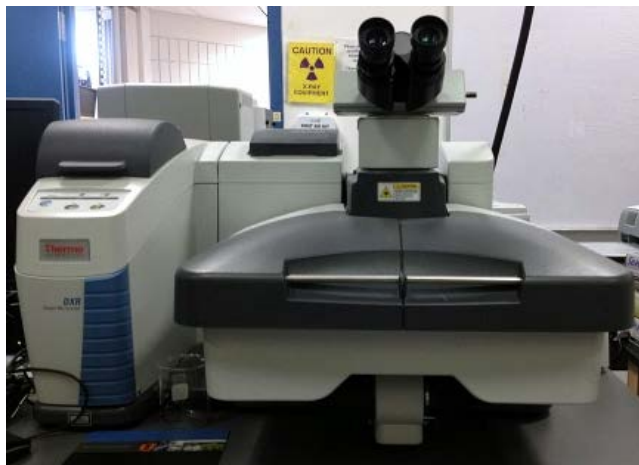
Figure 4: The dispersive Raman microspectrophotometer that was used in this research.
