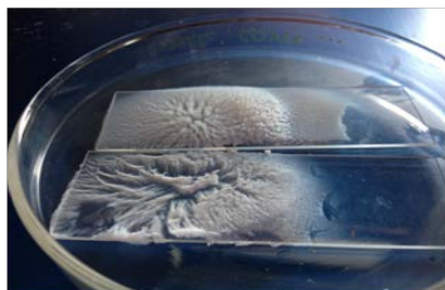
Figure 1. Silica nanofibers produced under the conditions of a 5 cm tip-to-collector distance, a 0.02 mL/hr flow rate, and an 11 kV voltage.
